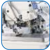
Presser foot arm with an open/close sensor
